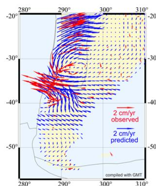
Top: DTRF2014, positions and horizontal velocities of geodetic observing stations.
