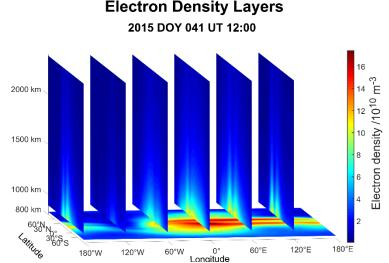
Estimated electron density distribution above 800 km altitude at February 10, 2015 at 14:00 UT, visualized by one horizontal layer at an altitude of 800 km and six vertical layers at different fixed longitudes
